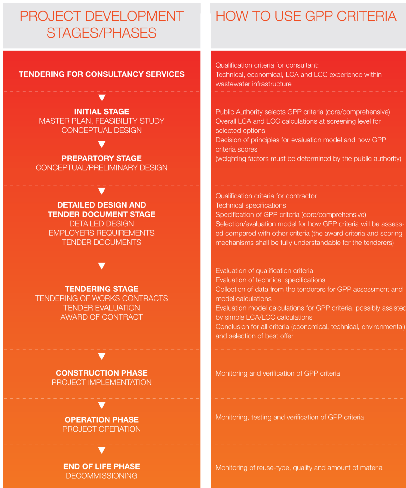
Figure 4-1 Project development and how to use GPP criteria in the different phases
